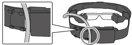
**3 Tighten the head band and secure the head pad.**
