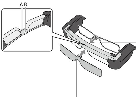
Install the shade or protective shield to the outside of the headset, and secure it in place using screw hole (A). You cannot install the shade and protective shield at the same time.
