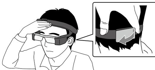
**Re-tightening Screws (BT-2000)**
