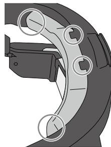
**Installing the Shade/Protective Shield/Lens Holder**
