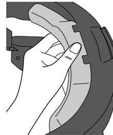
**2 Align the groove at the bottom of the replacement inner pad with the tabs on the headset.**
