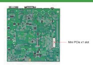
The WADE-8020 is built with the Intel® mobile QM57 chipset which works well with Intel® Core™ i5/i7 mobile processor technologies capable of supporting dual channel DDR3 memory. These features make the WADE-8020 the ideal solution for POS, Lottery, Medical, Gaming, High Resolution Digital Signage, Surveillance Security Monitoring, and Kiosk applications.
