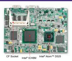
The PEB-2771/2781 takes advange of the latest Intel® Atom™ technologies. It supports DDR3 SDRAM, dual gigabit ethernet and one expansion Mini PCI Express x1 socket. Based on Intel® Atom™ solutions, the fanless PEB-2771/2781 executes high performance with low power dissipation. Therefore, it's applied to Panel PC, Kiosk, DS, Medical, Military and industrial automation.
