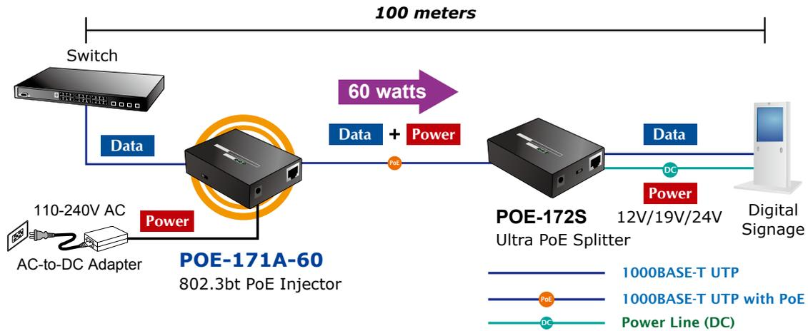
*Extended Installation of IEEE 802.3bt Injector and PoE Network*
