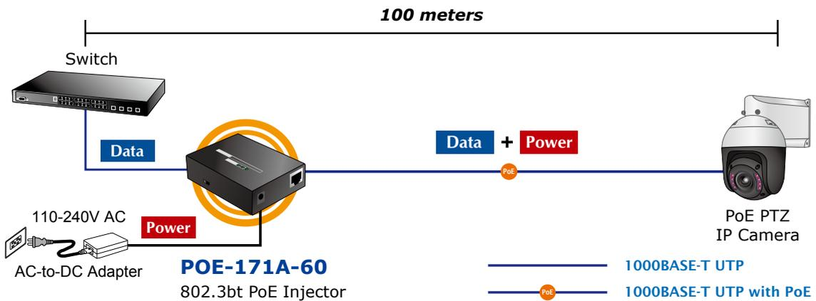
*Installation of 802.3bt PoE Injector and Splitter*
