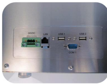
IP 54 Connector Ports Power Input, 3PIN, 24 V DC In, Phoenix 1 x RJ45, 2 x USB, RS232 D-Sub
